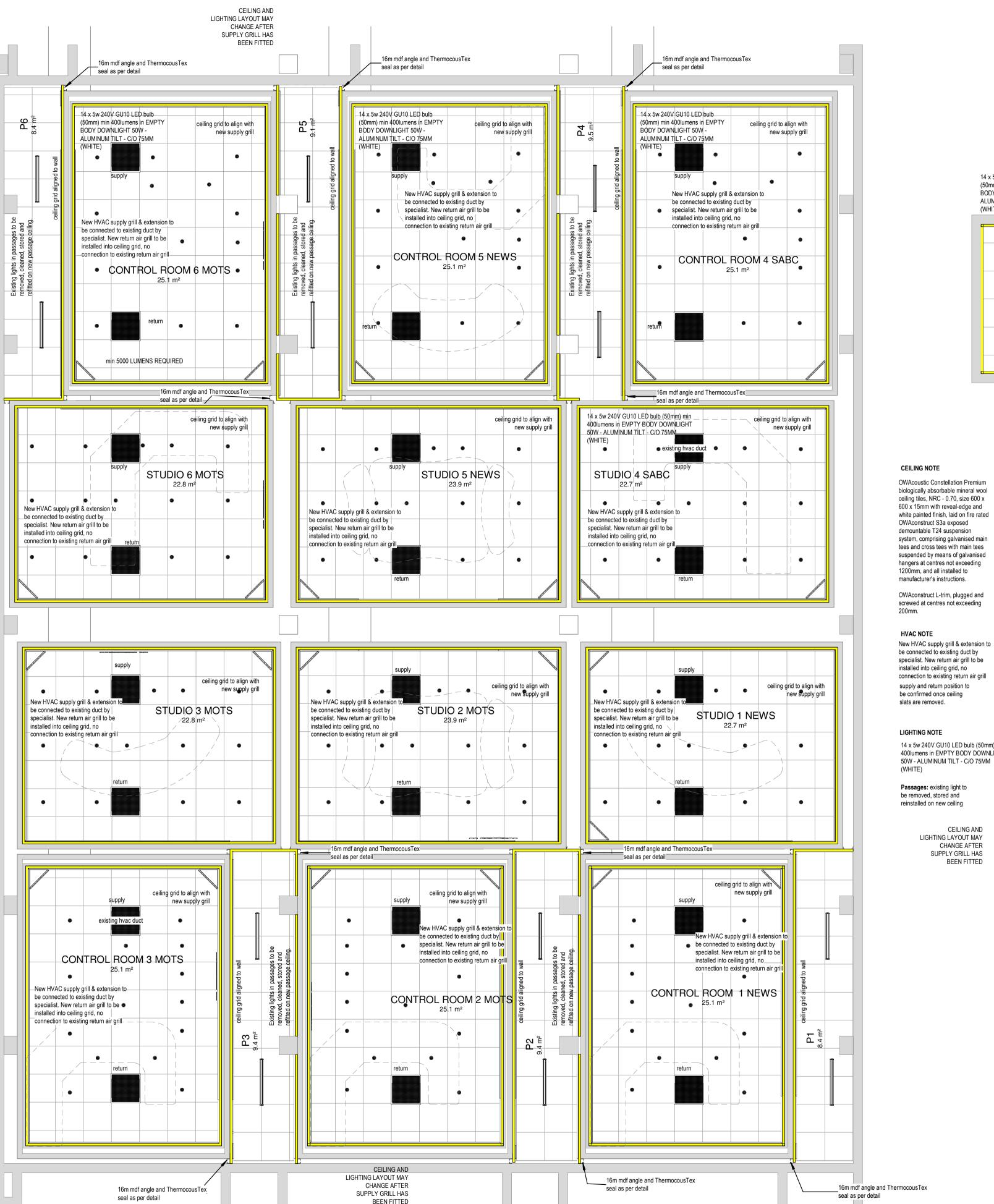
14 x 5w 240V GU10 LED bulb 14 x 5w 240V GU10 LED bulb (50mm) min 400lumens in EMPTY (50mm) min 400lumens in EMPTY BODY DOWNLIGHT 50W -BODY DOWNLIGHT 50W -ALUMINUM TILT - C/O 75MM ALUMINUM TILT - C/O 75MM (WHITE) ceiling grid to align with ceiling grid to align with new supply gril CEILING AND LIGHTING LAYOUT MAY CHANGE AFTER
